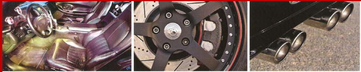
Above, left to right: Aside from some additional gauges, the interior is stock; iForged Aero wheels house upgraded brake rotors; Borla exhaust tips. Below: The big Procharger D15C supercharger sits in front of the engine. Opposite: Even the meaty 345-mm-wide Hoosier rear tires don't stand a chance against 710 lbs-ft of torque.
